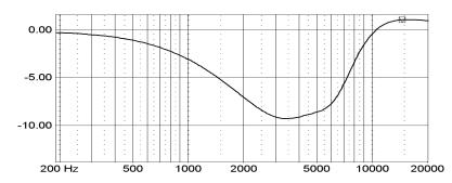
F1=3.43khz, -9.1dB, Q=0.79, BW=1.27 Oct F2=5.76khz, -6.1dB, Q=1.49, BW=0.67 Oct F3=11.3khz, +5.55dB, Q=1.24, BW=0.8 Oct
