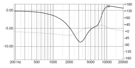
F1=3.25khz, -9.0dB, Q=1.37, BW=0.73 Oct F2=6.47khz, -3.15dB, Q=2.5, BW=0.4 Oct F3=9.77khz, +2.9dB, Q=1.2, BW=0.82 Oct
