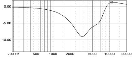
F1=3.4khz, -9.3dB, Q=1.4, BW=0.71 Oct F2=6.42khz, -7.6dB, Q=1.47, BW=0.68 Oct F3=9.48khz, +6.4dB, Q=1.19, BW=0.84 Oct
