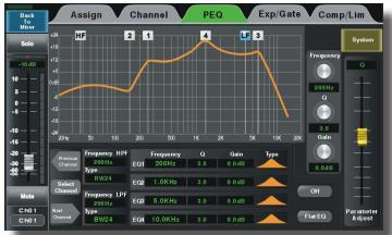
Figure 4.2: PEQ Parametric EQ Screen
