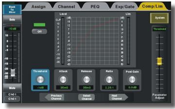
Figure 4.5: Compressor/Limiter Screen
