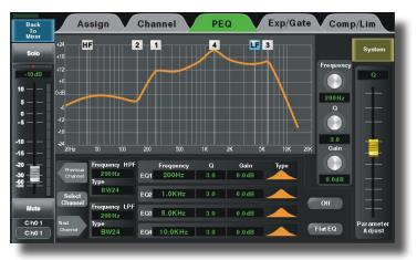
Figure 4.2: PEQ Parametric EQ Screen
