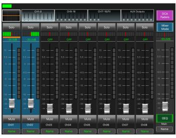
Figure 4.6a: Ch1-2 stereo linked, Long Fader mode
