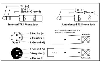
3.1 - Balanced and Unbalanced connector wiring
