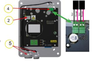
The cables must secured with the supplied tie-wrap (5) to prevent any stress on the terminal block.
