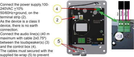
In « wired mode » (dip switch 2 in the OFF position) the power supply of the Melodys is what controls the ringing programmed by the master clock. The melody selected in the Melodys is played whenever the circuit is closed by the master clock.
