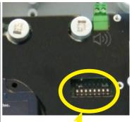
Beware: in DHF version the DIP switch 2 must be in the ON position.
