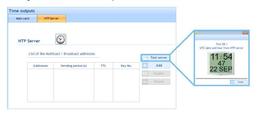
In NTP server mode, the master clock sends the time to the selected IP addresses with the selected mode of transmission.
