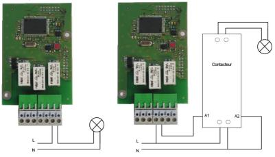
For relay circuits provide protection by disconnecting the fuse or circuit breaker maximum 4A. Please indicate on the terminal label the location of these protections.
