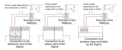
The Melodys can be connected directly to a relay output of the master clock, an option card or a wireless relay.
