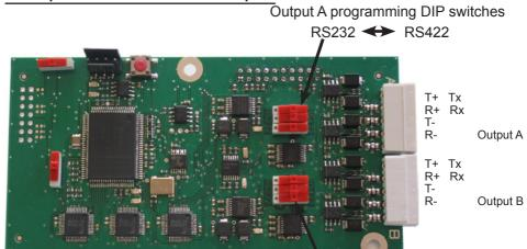
Output B programming DIP switches
