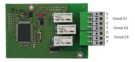
This option board does not require any software programming. It allows 3 relays to be added.
