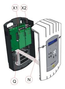
**<u>RACK version</u>** : Open the rack unit and install the option board(s) in the slots provided (X1) to (X2).
