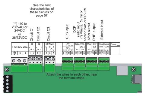
(\*) See page 33, the "Time outputs" menu to set this output (Pulse minute,  $\frac{1}{2}$  minute, second 24V or power TBT 24VDC 1A).
