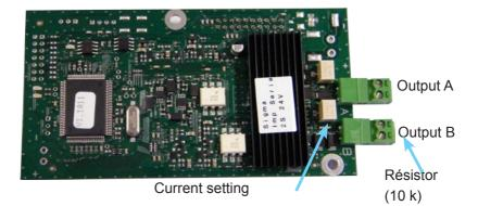
This option board does not require any programming. By default the time is the local time defined in the Sigma, with 1.2-second impulses, and the line is stopped.
