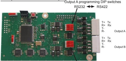
Output B programming DIP switches RS232 ↔ RS422
