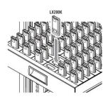
Step 5: LEDs on the charger flash 5 times, indicating synchronization is taking place
