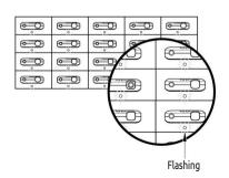
Step **6**: LEDs turn to solid and now indicates the battery charging status. The synchronization process is completed and you are ready to use your system.
