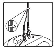
**10.** Use zip or twist-lock ties to secure safety cable & signal wire to main hanging cables. Cable cover available for asthetic applications (SLT-10).
