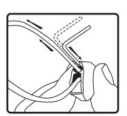
**7.** Adjust speaker hanging height with SpeedClamp<sup>™</sup> mechanism. Pull to tighten & insert release key (small hex wrench) into SpeedClamp <sup>™</sup> as shown to loosen or adjust.
