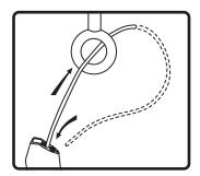
**5.** Attach the hanging cable by securing it and the safety cable to structure as shown.
