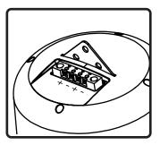
2. Connect signal wire to screw-down terminal block. Tighten unused terminal screws. Use inside positive and negative inputs for either voice coil or distributed systems.
