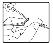
**6.** Thread cable end(s) through SpeedClamp<sup>™</sup> mechanisms as shown.
