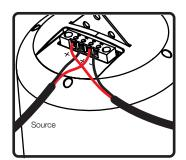
**3.** When daisy chaining, wire the outside terminals to the inside terminals of the next speaker. This step only applies to tap settings using the transformer and not when the speaker is used on bypass.
